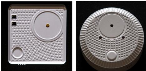
WG's audible/visual remote alarm sounds once an attempt or an attack has been made to the smart tag. This remote can detect an attack on a tag up to 40 ft away via WG's smart technology.
