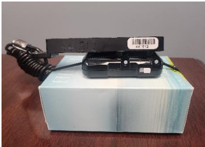
Align the ears of the detacher with the indentations on the tag.
