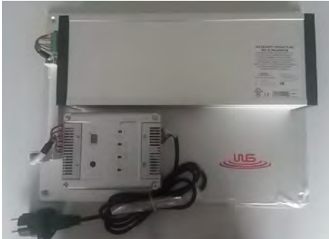
System controller with SPS Smart Power supply on the mounting plate
