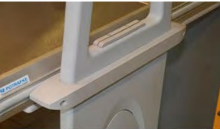
At Tandem cash desk's the antenna is centered between the lanes and is attached by the FS kit to the customer guiding elements (eg Wanzl).
