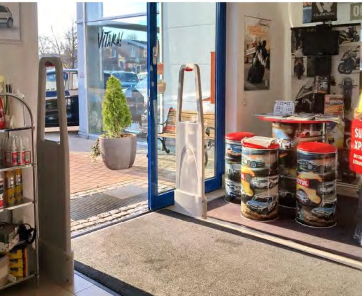
The durable ABS body of Lane Guard makes it enormously robust. A dual configuration can protect a free entrance of 5ft - 6ft using labels or small hard tags.
